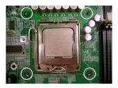
4. Press the heatsink down until the four screws are securely seated in the holes.
